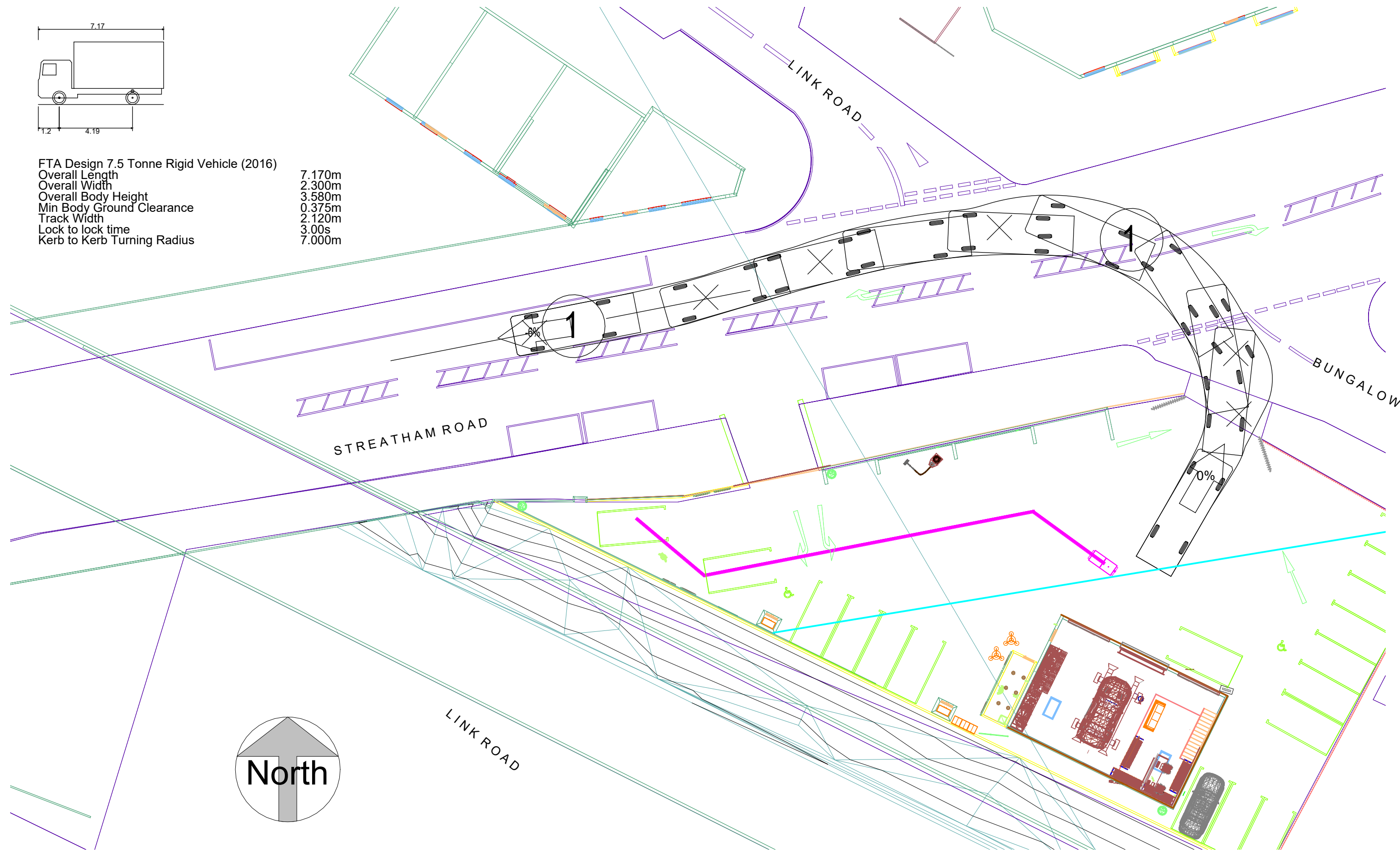
SWEPT PATH ANALYSIS ON EXITING 225 STREATHAM ROAD SITE AND TRAVELLING SOUTH WEST DOWN STREATHAM ROAD. SCALE 1:200
